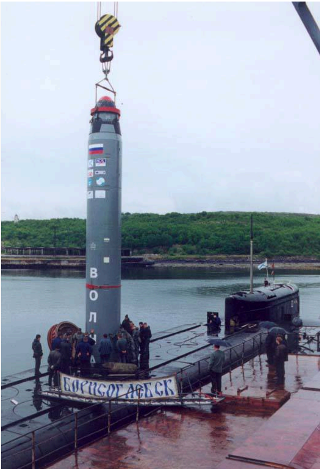
Loading the R-29R missile into the silo of the K-496 Borisoglebsk submarine (decommissioned in 2009). Photo Warfare.be
